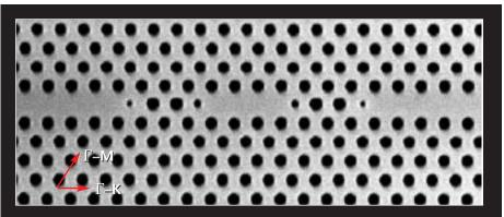
**Figure 6**. Three-point defect in a silicon photonic crystal forms a microcavity that catches resonant light. [Postdeadline paper QPDA5, Figure 1b.]
